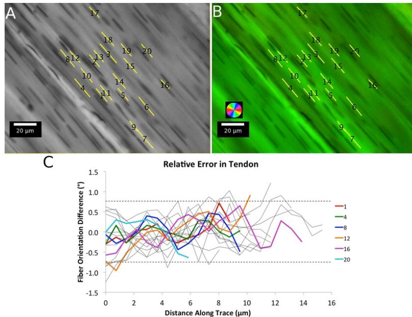
Fig. 4. Accuracy in loaded tendon tissue. Using images of loaded tendon (A), we compared PLM orientation (B) with orientation of manual traces. The relative error was small for all 20 traces (C). For clarity, six traces were highlighted in color, with the rest shown in grey. The dotted lines represent the 2.5th and 97.5th percentiles of the orientation differences.
