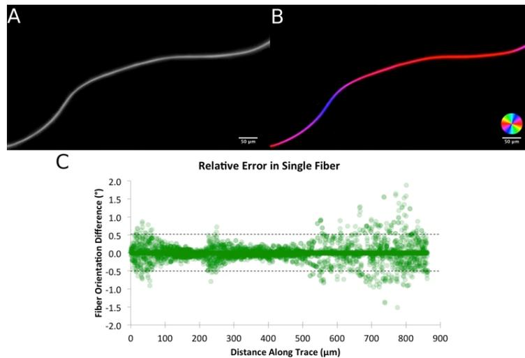
Fig. 5. Accuracy in a single curved silk fiber. Using images of a single curved silk fiber (A), we compared PLM orientation (B) with the interpolated orientation along a curved manual trace. The relative error was small along the entire trace (C). The dotted lines represent the 2.5th and 97.5th percentiles of the orientation differences.
